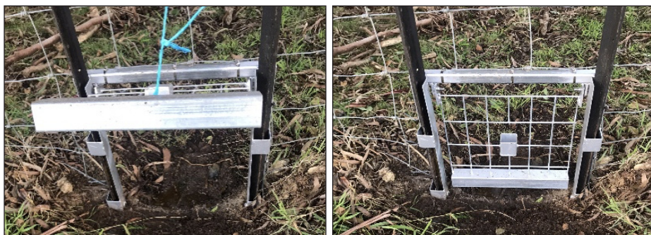
Wombat swing gates are easy to install and should be placed on well-used wombat tracks. Installation is simple and instructions are provided. Once installed, it is best to tie the gate up for a couple of weeks so the wombats slowly get used to the change in the fence. The gate is then lowered.
