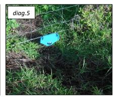
A wire frame is positioned at the entrance to the burrow. A distance of 30cm from bottom of flap is ideal and means the wombat just has to duck its head to go under. Make sure the cable ties are pulled tight to stop the flap from moving around on the wire frame but be sure the flap can move forward & back without disturbance (*diag.3*). The wire frame can also be pushed into the top of the burrow (*diag.4*).
