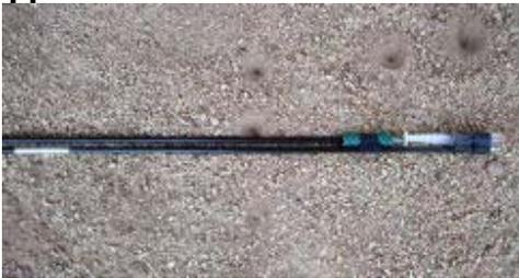
We've used fibreglass tent poles as these fold up and are light. Using hose tube as a guide a second tent pole is lined up with the syringe plunger allowing around three metres of reach.
